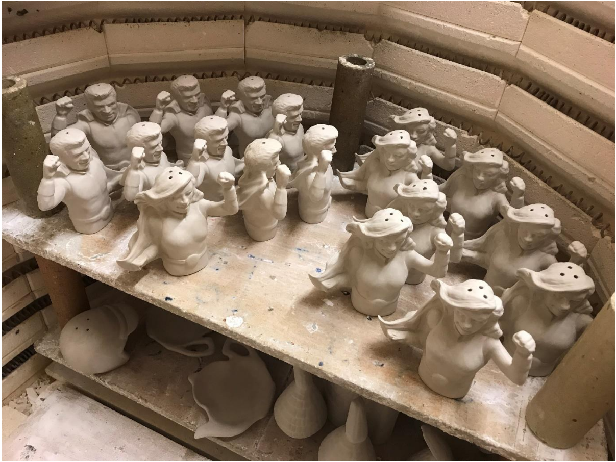
The first heroes coming out of the kiln after their biscuit firing. Now ready for painting.
